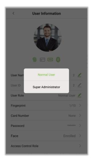
**Note:** When a user is given Super Administrator privileges, verification is required to open the main menu. The verification process depends on the verification method that was used during user registration. See the description in section <u>Verification Modes</u>.
