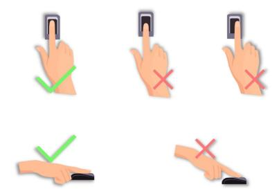
Note: Please press your fingers onto the fingerprint reader firmly for registration and identification.
