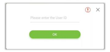
If a user has registered a Face, Fingerprint and Card in addition to his/her password and the verification method is set to Fingerprint/ Password/ Card/ Face verification, the following screen will appear. Select the password icon (a) to open password verification mode.
