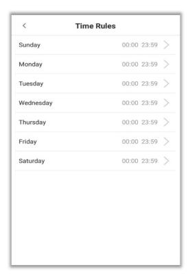
Tap the date on which time rule settings is required. Set the starting and ending time, and then press **[OK]**.
