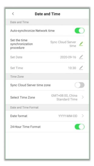
**Auto-Synchronize Network Time:** Enabled by default, and the device synchronizes the current Network time. If disabled, the user can set the date and time.
